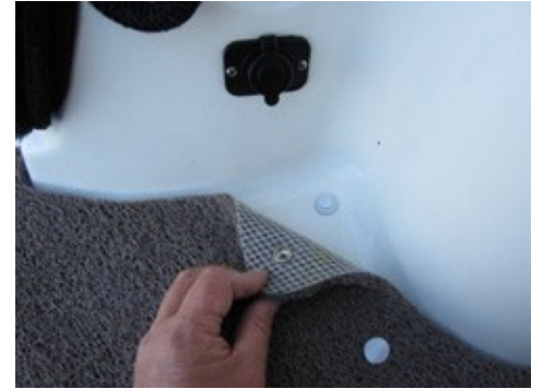
Male is attached to deck with no holes
